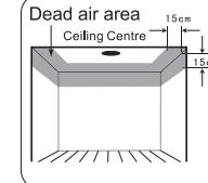
The preferred location to install the smoke detector is in the centre of the ceiling because smoke, heat and combustible products rise to the ceiling and will laterally spread. Keep at least 30 cm distance from lights and decorations and at least 15 cm distance from walls and corners.
