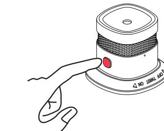
To test or to mute the alarm, press and hold the Test / Mute button for 3 seconds.
