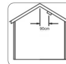
Please install the smoke detector at 90 cm horizontal distance from the ceiling top.
